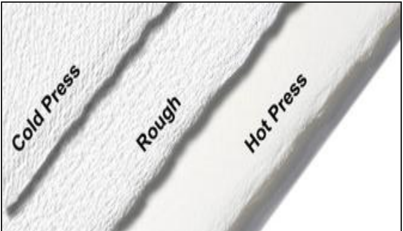
Difference in the textures of Hot- pressed, Cold-pressed and Rough Paper
